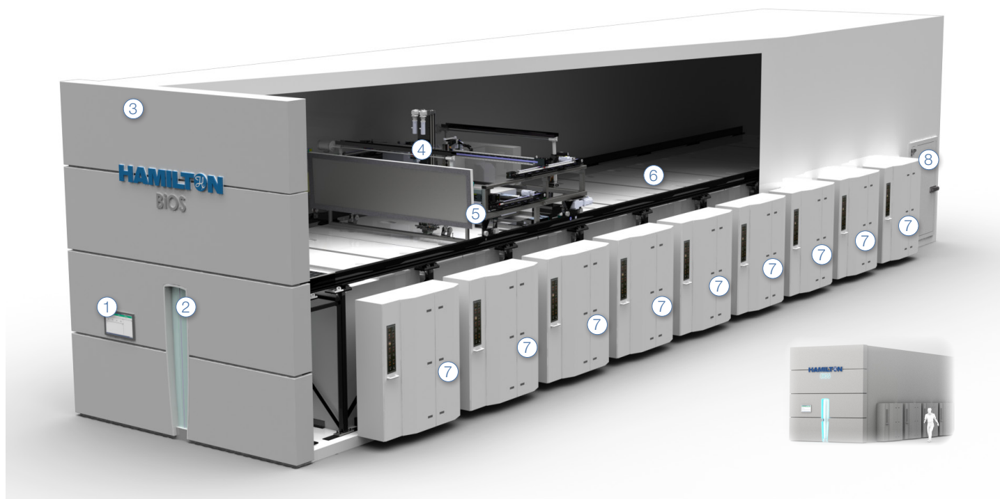
Figure 4: Main Features of the BIOS® automated storage system. (1) Graphical User Interface, (2) User Access, (3) System Enclosure, (4) Internal Robotics at -20°C, (5) -80°C Tube Picker, (6) -80°C Storage Compartments, (7) Refrigeration Systems (freezers), (8) Service Access. The figure at the bottom left offers a perspective of the size of the system in comparison to the size of an average adult.
