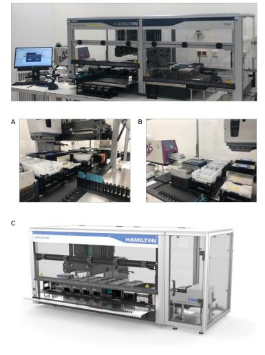
**Figure 2.** Automated library preparation on the Hamilton STARplus with (A) 96well pipetting heads, (B) on-deck thermocycler and (C) Covaris R230 Focusedultrasonicator.
