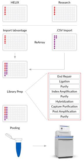
**Figure 1.** Experimental diagram of the library preparation workflow on the Hamilton STARplus. 32 samples are processed per run, with the ability to increase to 64 samples.
