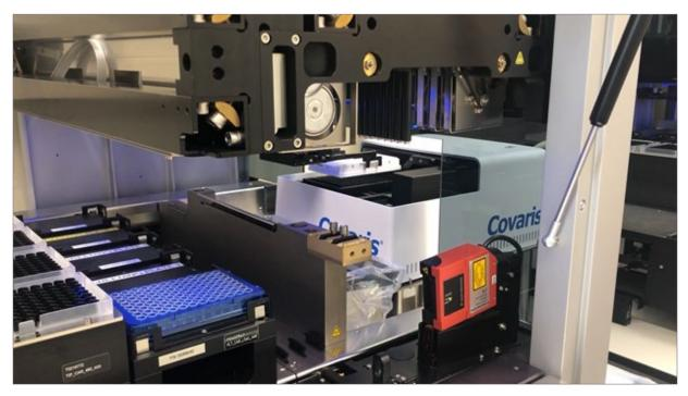
Figure 3. Picture of the R230 Focused-ultrasonicator integrated on deck with the Hamilton STARplus. This R230 is integrated onto the deck of the STARplus used for sample normalization
